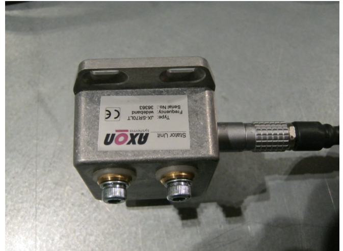
Photograph 2.3-6: Example of an Axon Stator Unit used for the antenna connection
