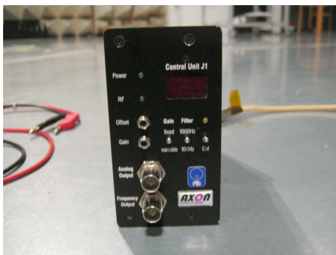
Photograph 2.3-3: Axon System Control Unit J1 CS10, front view
