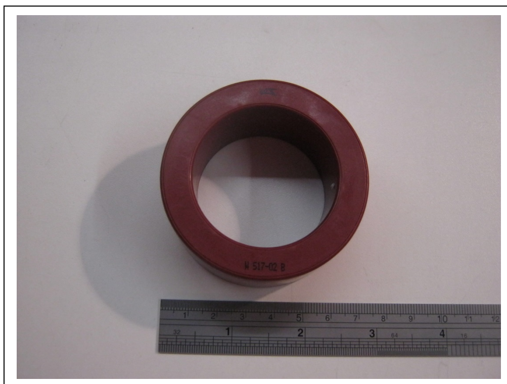
Photograph A3-6: Detail on ferrite VITROPERM 500F, Type T60006-L2063-W157
