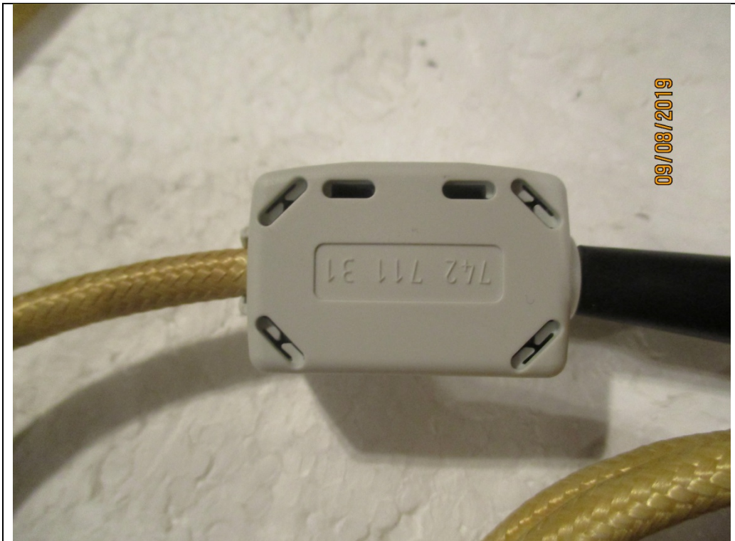
Photograph A3-5: Detail on ferrite Würth 742 711 31 at connector to the Axon control unit
