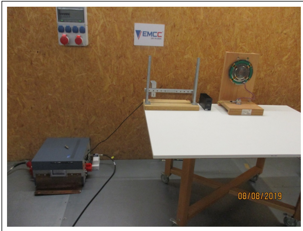
Photograph A1-1: Conducted emissions
