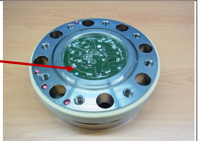
The rotor includes 4 PCB*
