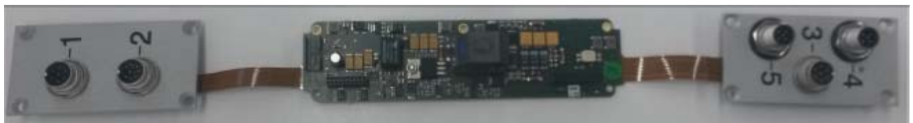
Supply - Interface PCB front side*
