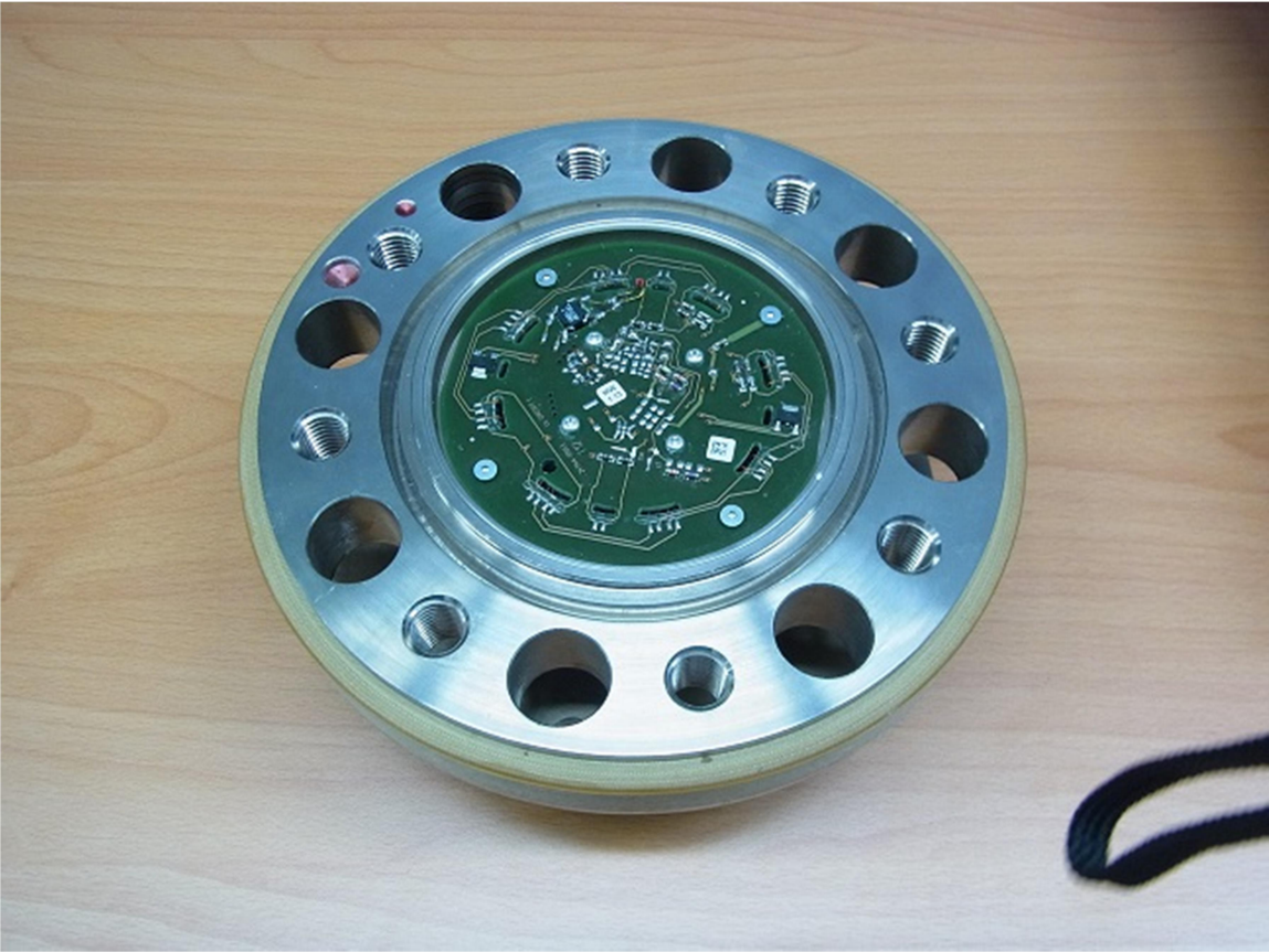
The rotor includes 4 PCB
