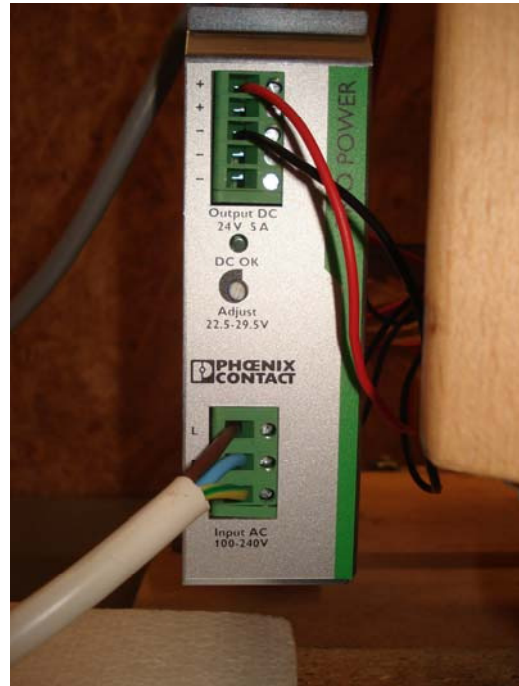
Photograph 2.3-2: Power supply TRIO-PS/1AC/24DC/5, front view
