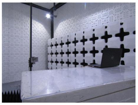
Conducted disturbance voltage at mains ports (150KHz-30MHz)
