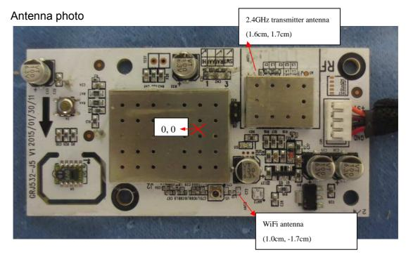
The power densities of up to 2 antennas located within a 16 cm<sup>2</sup> region at 0.1cm intervals are estimated first. Then the power densities computed for each antenna are summed.
