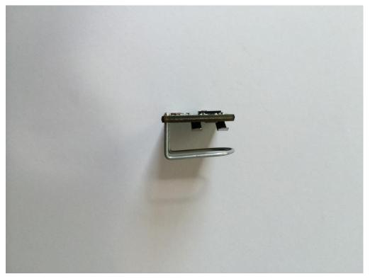
Metal structures on the bottom are for holding the battery in place. It is a positive and a negative connection.
