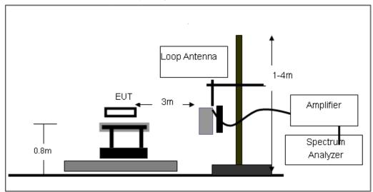
(B) Radiated Emission Test-Up Frequency 30MHz~1GHz
