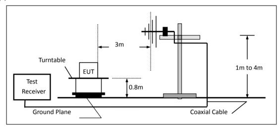
(c) For radiated emissions above 1000MHz
