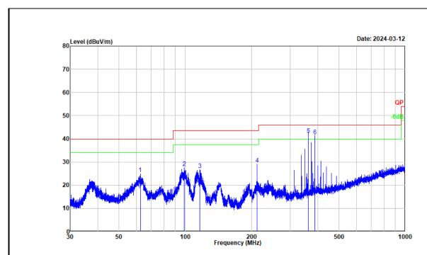
Project No. : RWAQ202400235 Test Mode : Transmitting Test Voltage : DC 5V
