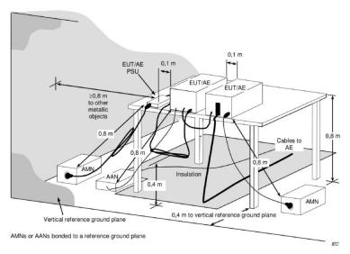
**Note:** The 0.8 m distance specified between EUT/AE/PSU and AMN/AAN, is applicable only to the EUT being measured. If the device is AE then it shall be >0.8 m.
