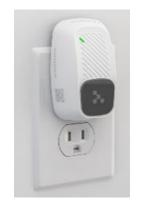
The Portal Light 2 is Kontakt.io's Bluetooth® Low Energy (LE) gateway device. It scans and detects Kontakt.io BLE devices and sends received BLE data to Kio Cloud over the facility's existing Wi-Fi network. With a Kontakt.io subscription, BLE beacons, tags, and badges are automatically processed in Cloud and Applications and can receive configuration/firmware updates over their BLE connection to a Portal Light 2.
