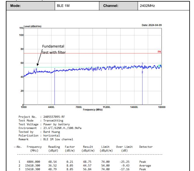
Remarks: Factor = Antenna factor + Cable loss - Preamp gain
