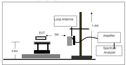
(B) Radiated Emission Test-Up Frequency 30MHz~1GHz
