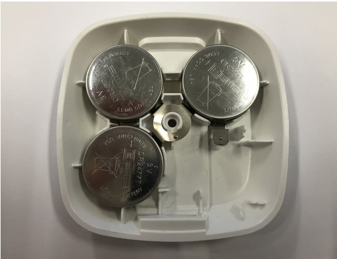
Casing base with batteries
