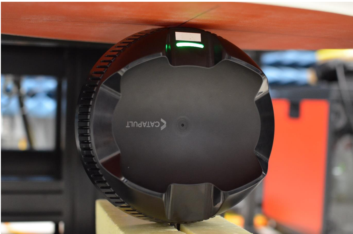
SAR Test Setup Photo 4: Body, Top Edge, 0 mm
