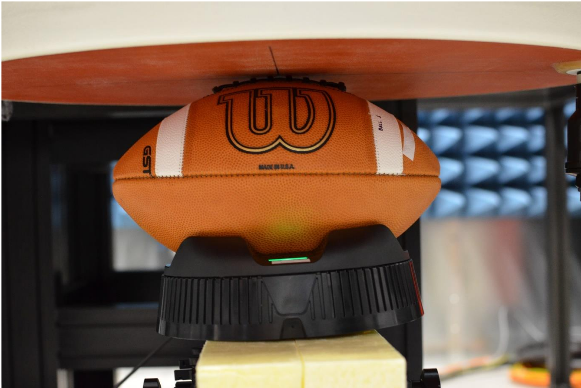
SAR Test Setup Photo 1: Body, Client Device on Cradle - Laces Up, 130 mm
