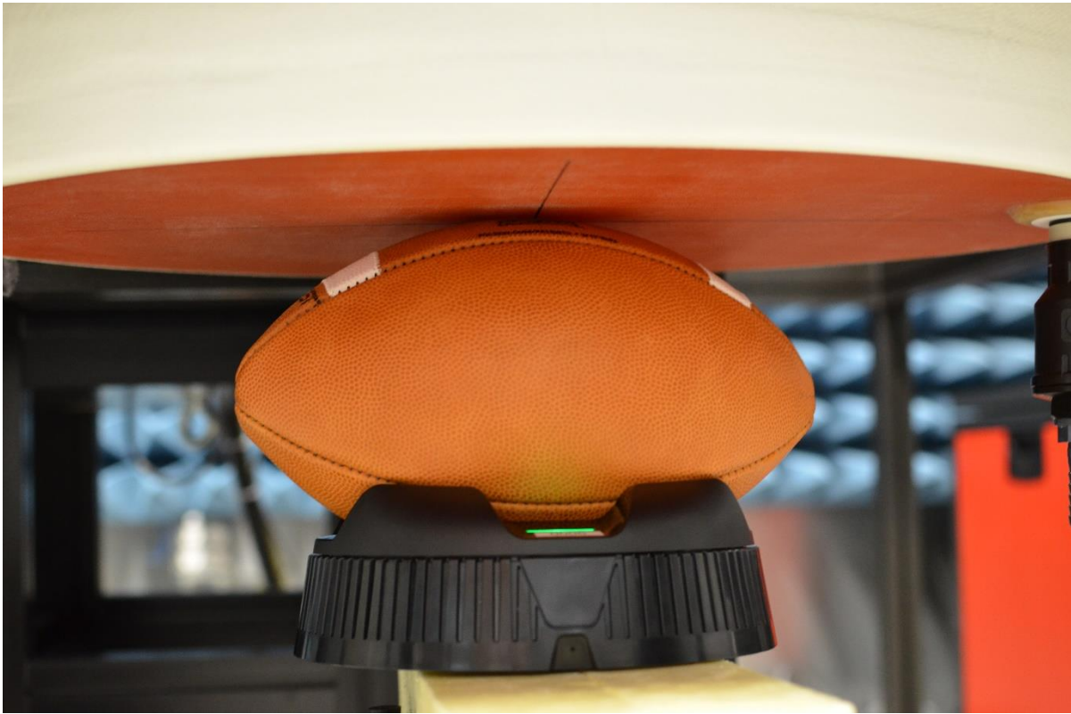
SAR Test Setup Photo 3: Body, Client Device on Cradle - Air Hole Up, 130 mm
