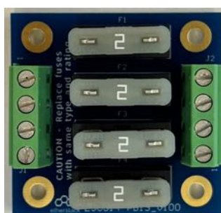
Photo 17 – PB13 Fuse Board Assembly Top View
