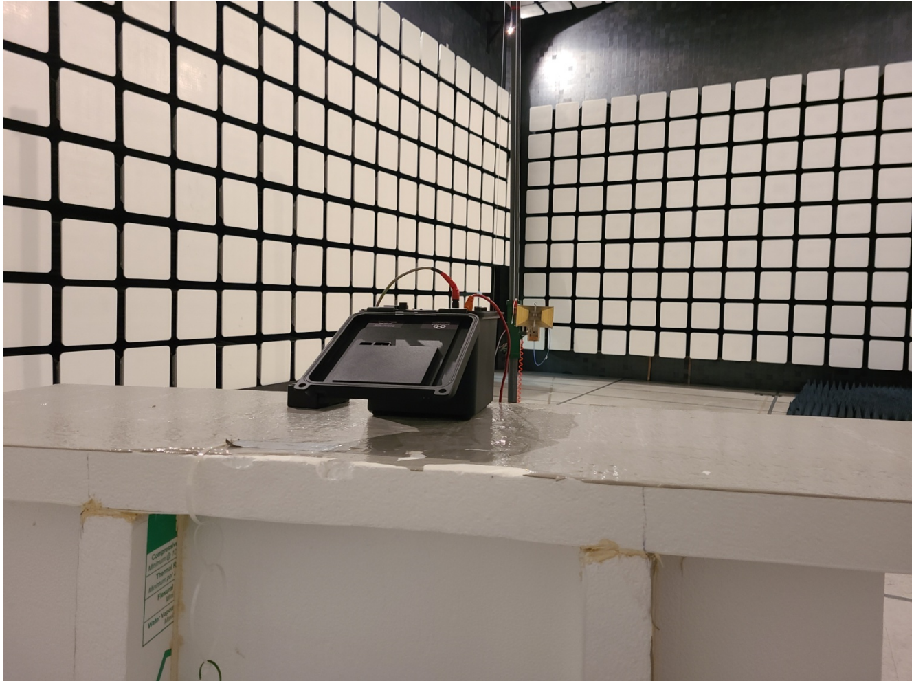
Test Configuration 1 Radiated Emissions at 3 m, Above 1 GHz
