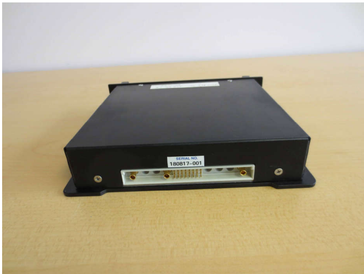
Photo 2: Internal Duplexer Module – With Cover – Connector End
