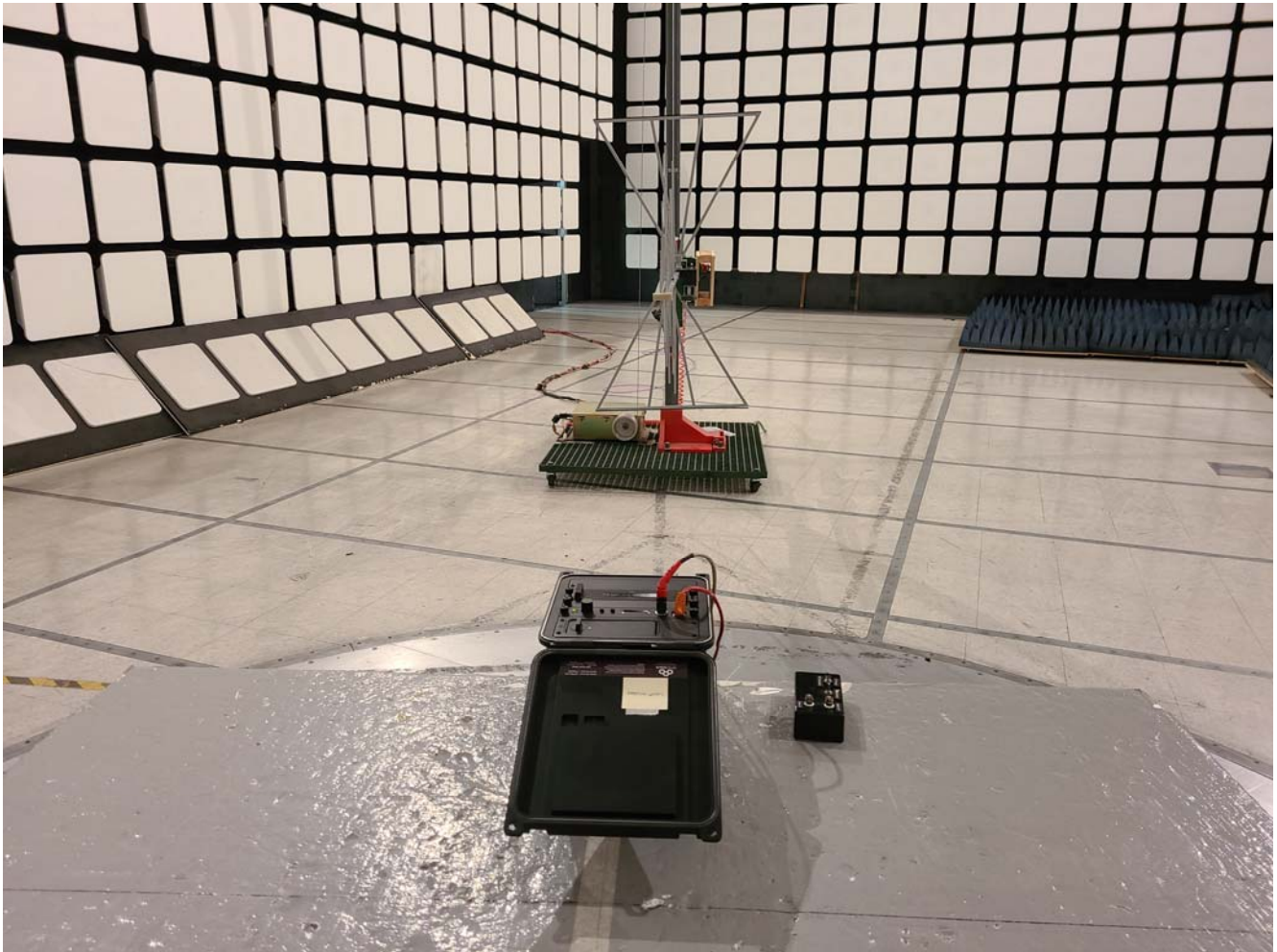
Test Configuration 1 Radiated Emissions at 3 m, 30 - 1000 MHz
