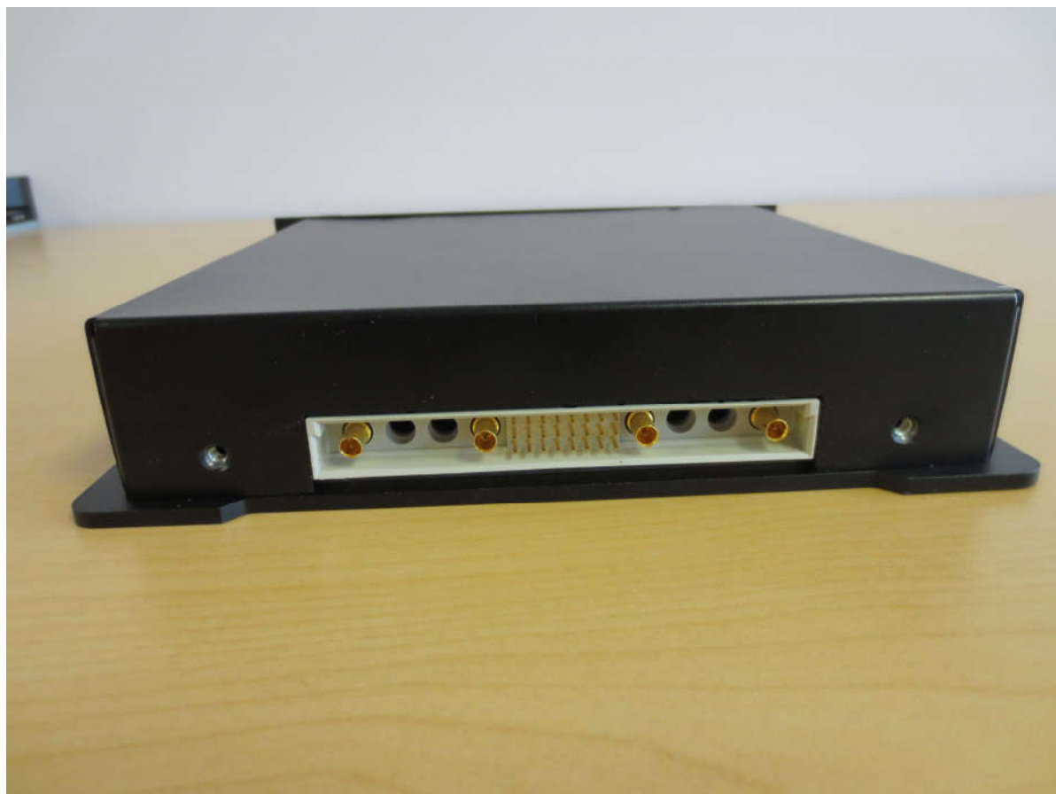
Photo 8: Duplexer Bypass Module – With Cover – Connector End
