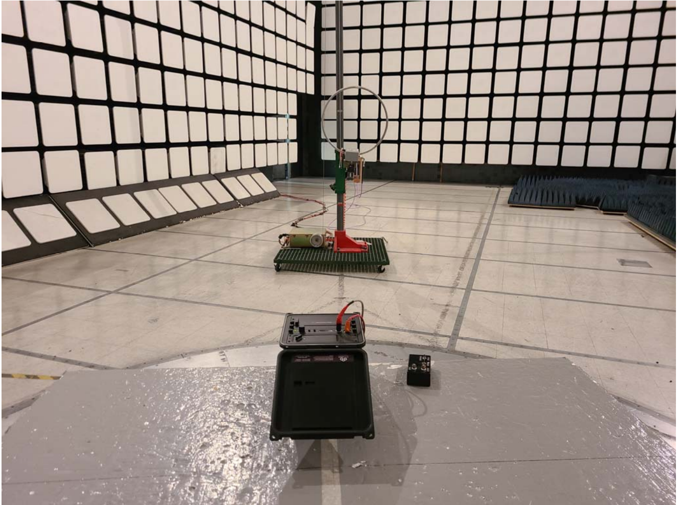
Test Configuration 2 or 3 Radiated Emissions at 3 m, 30 - 1000 MHz
