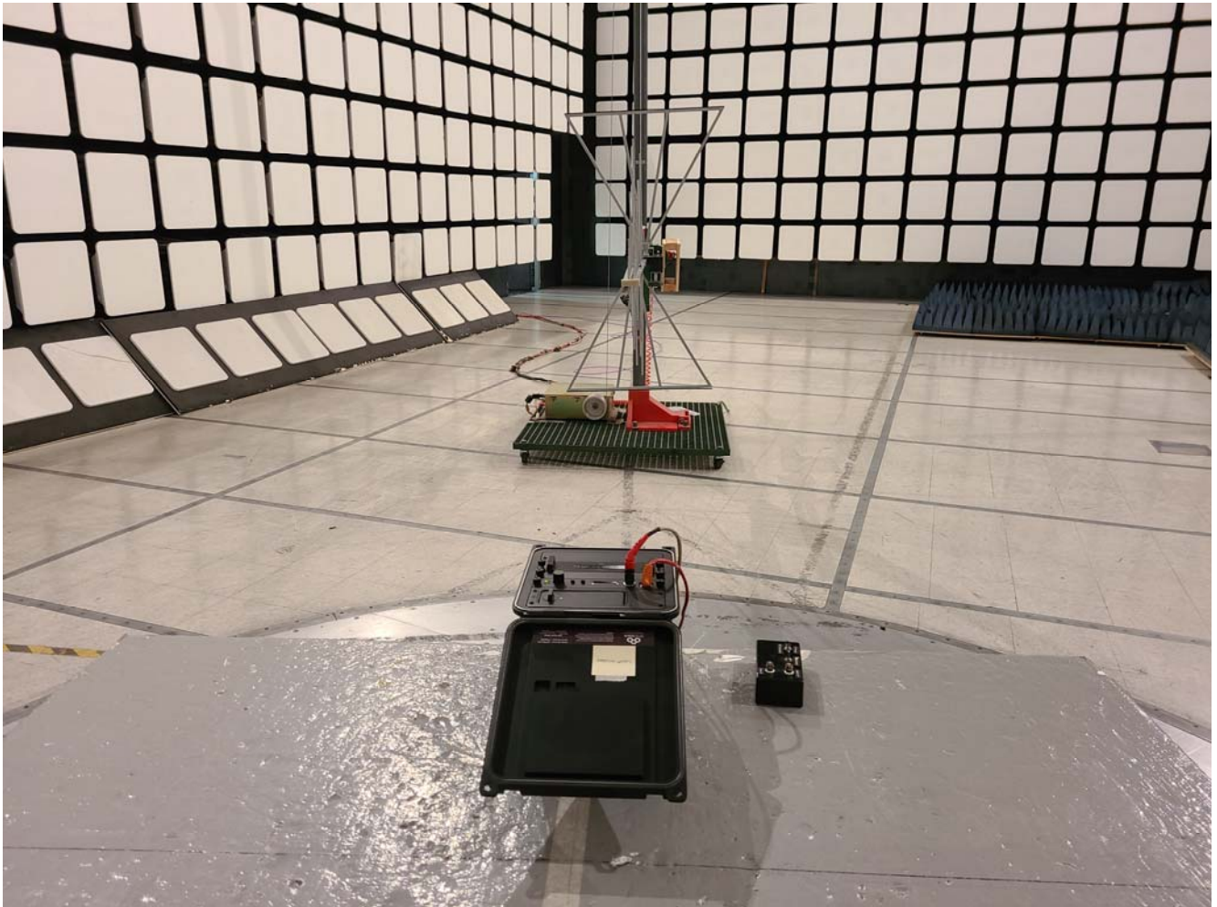
Test Configuration 1 Radiated Emissions at 3 m, 30 - 1000 MHz
