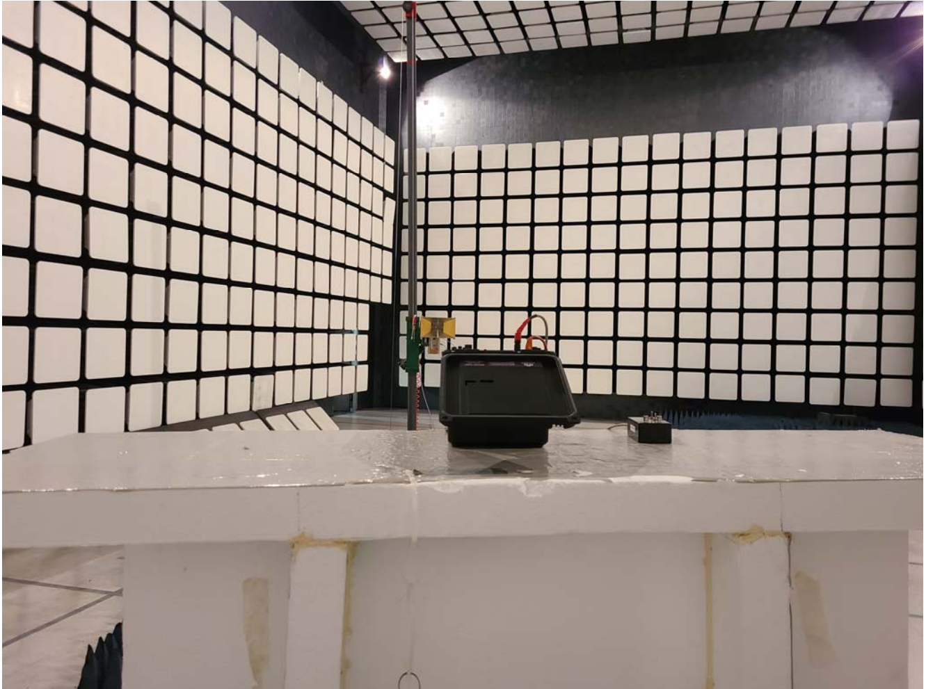
Test Configuration 2 or 3 Radiated Emissions at 3 m, Above 1 GHz
