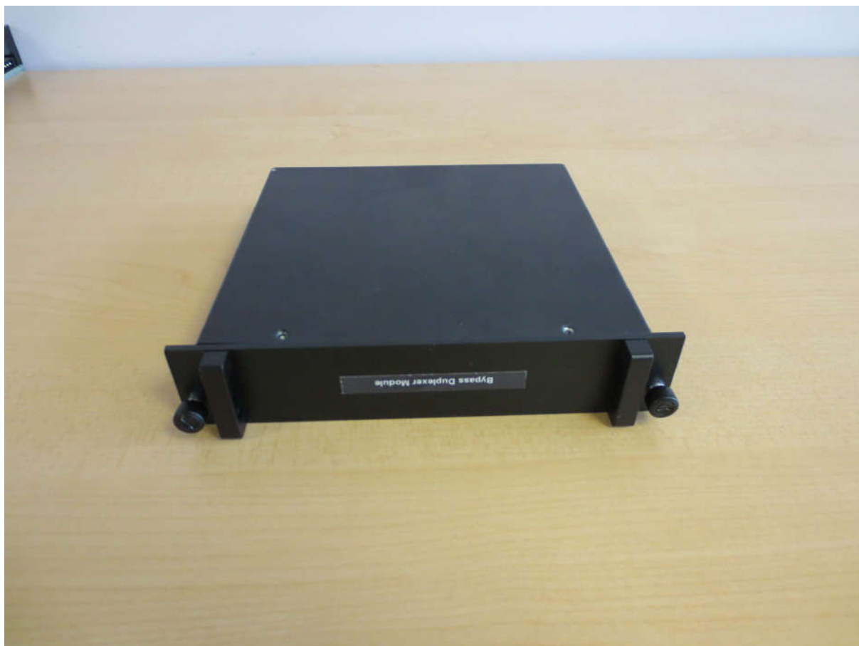
Photo 7: Duplexer Bypass Module – With Cover – Top End
