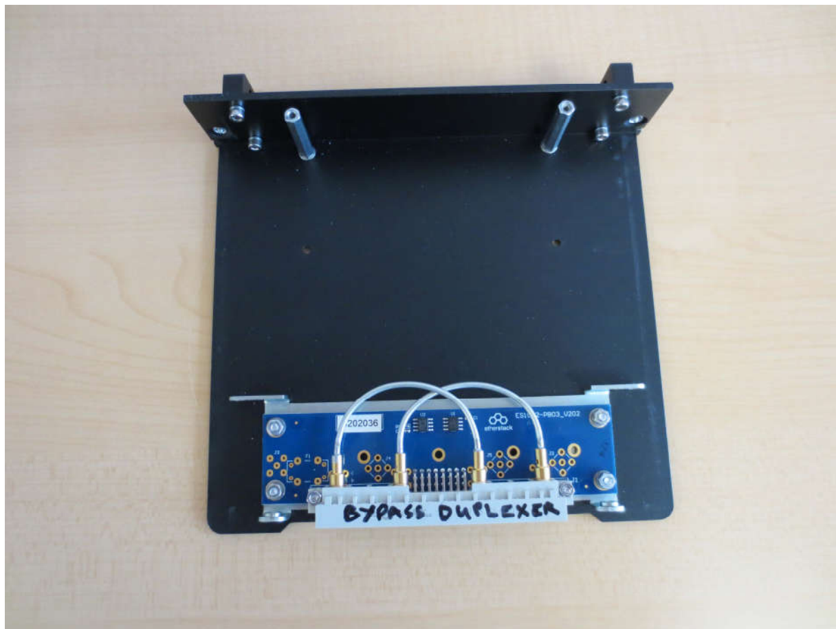
Photo 10: Duplexer Bypass Module – Without Cover – Top
