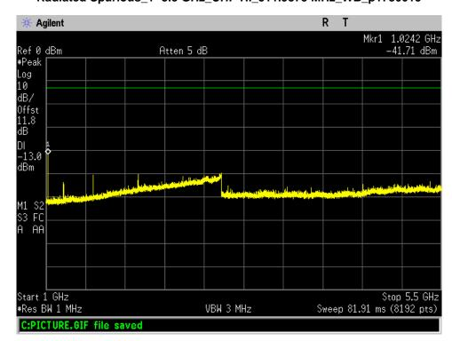
Radiated Spurious\_1- 5.5 GHz\_UHF-HI\_Standby\_p1780015
