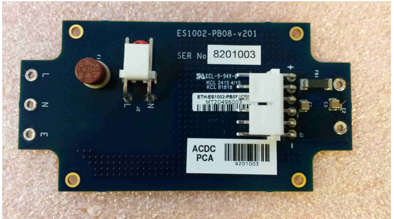
ES1002-PB08 AC/DC PCB Assembly Top
