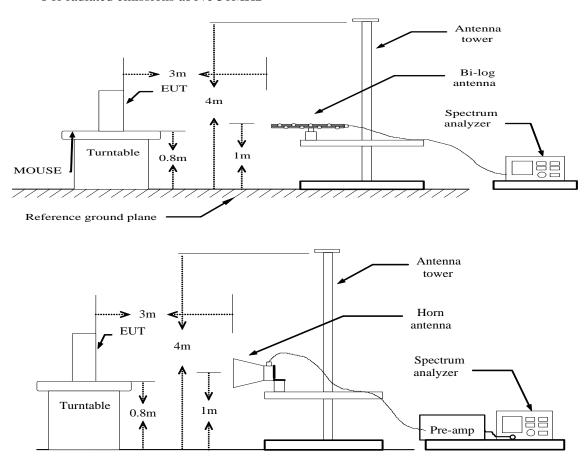
Above 10 GHz shall be extrapolated to the specified distance using an extrapolation factor of 20 dB/decade form 3m to 1.5m.
