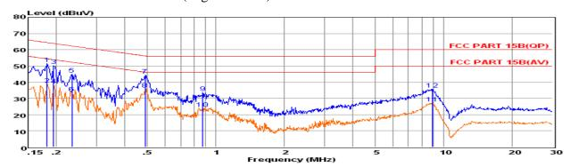
Env. Ins: EUT: M/N: Power Rating: Test Mode: Operator: 24\*/56% Media hub for Android NEO X8H Plus AC 120V/60Hz 802.11b-High channel Jacky
