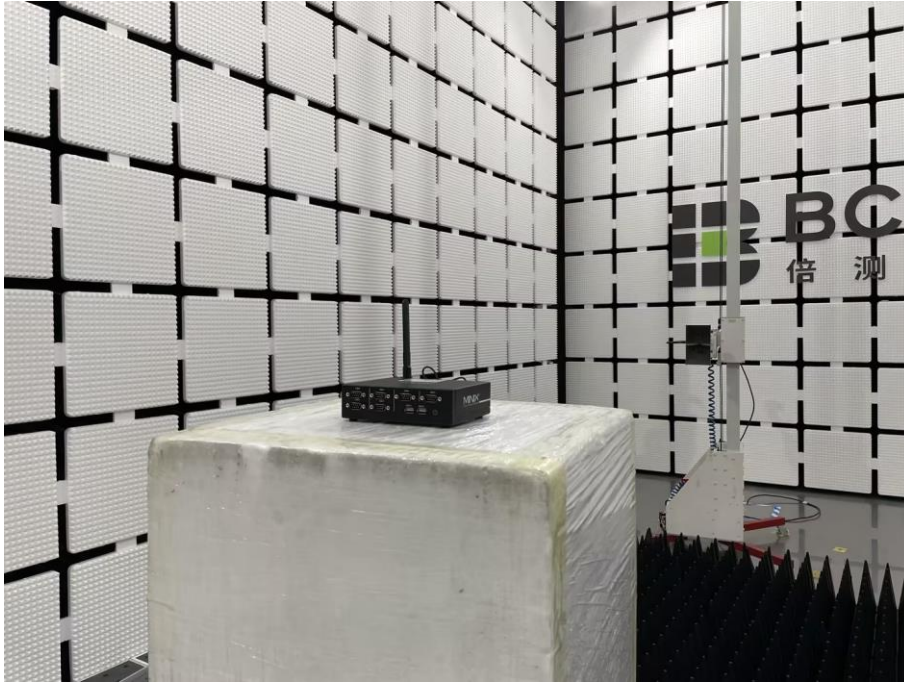
Spurious Emission Test Setup (Above 1GHz)
