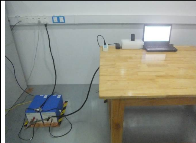
Conducted Emissions Test Setup – Front View
