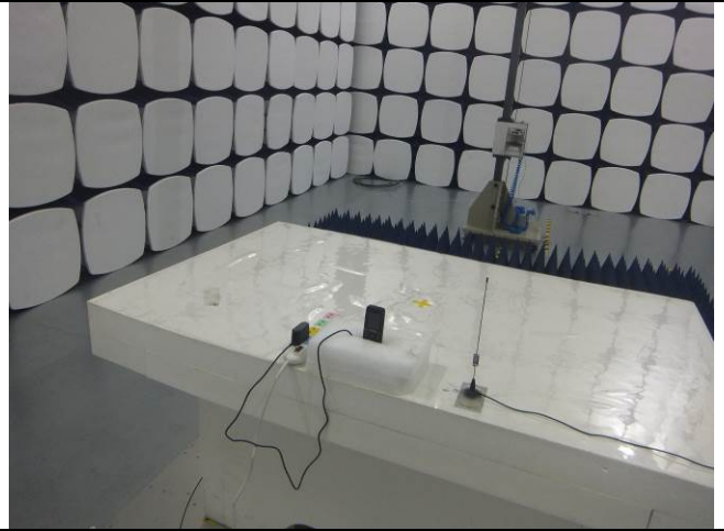
Radiated Spurious Emissions Test Setup Above 1GHz
