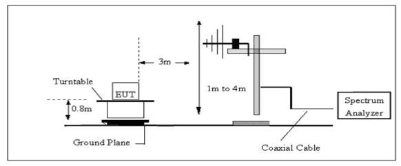
(A) Radiated Emission Test-Up Frequency 30MHz~1GHz
