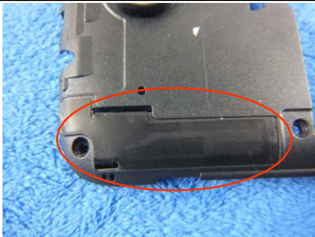
LTE - Antenna View
