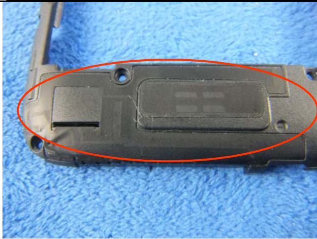
GSM/PCS/UMTS-FDD Antenna View
