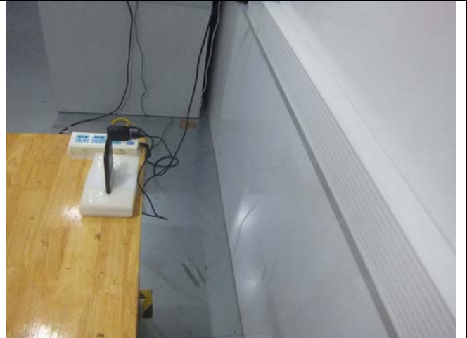
Conducted Emissions Test Setup Side View
