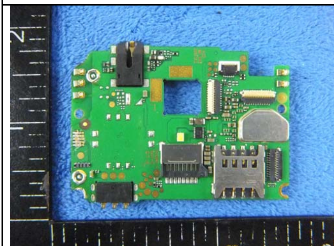
Mainboard with Shielding - Front View
