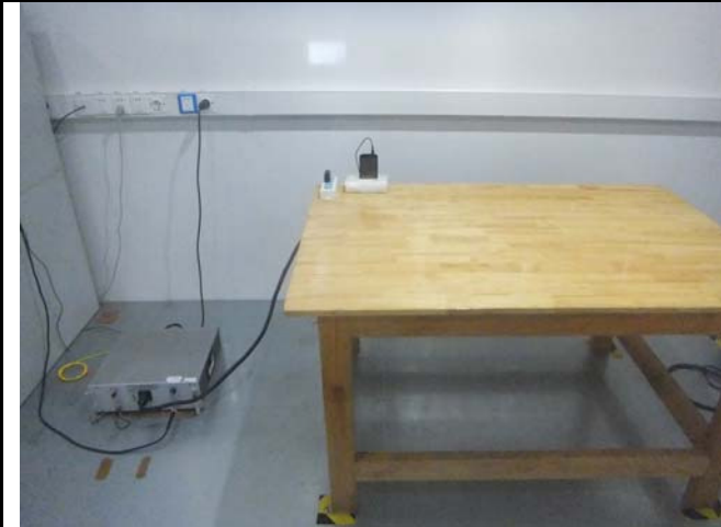
Conducted Emissions Test Setup Front View
