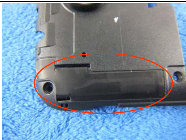
LTE - Antenna View
