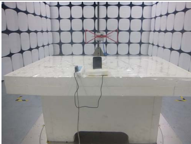
Conducted Emissions Test Setup Front View
