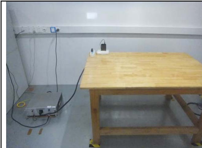
Conducted Emissions Test Setup Front View
