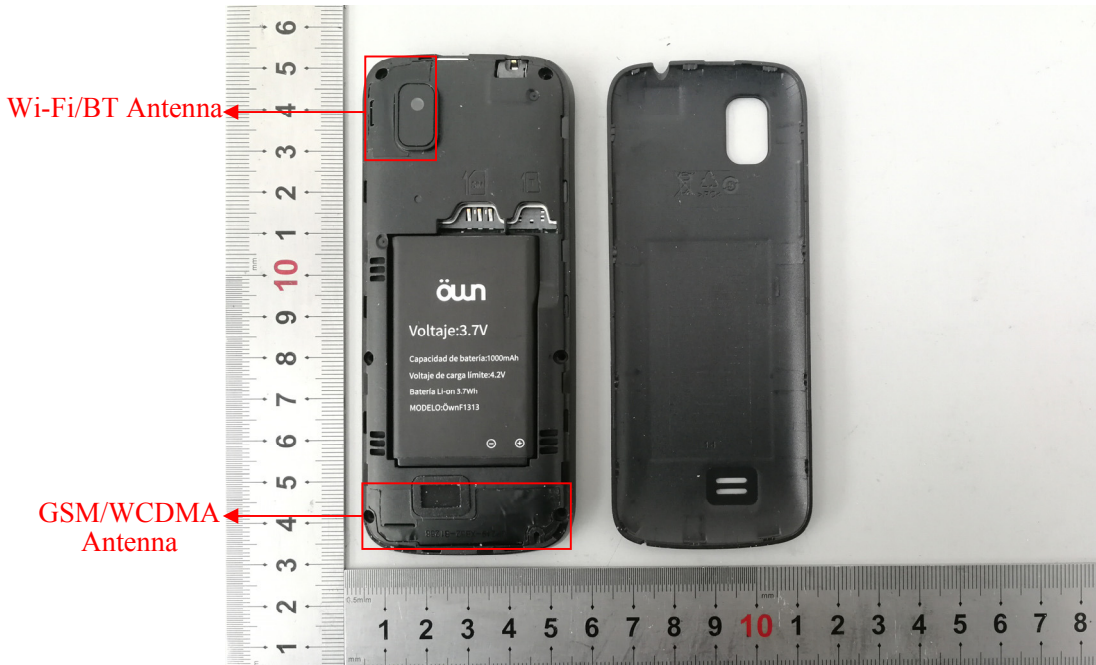
EUT – Cover off View-2
