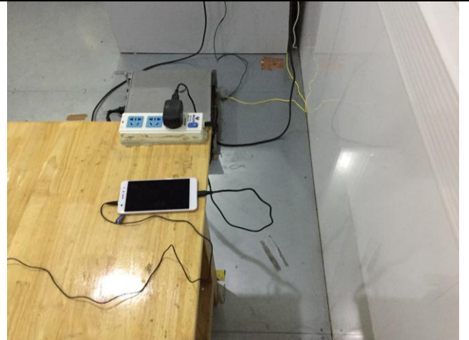
Conducted Emissions Test Setup Side View
