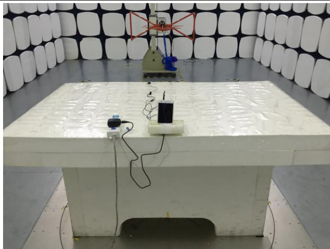
Conducted Emissions Test Setup Front View
