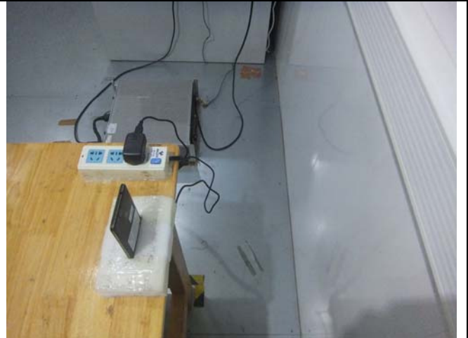
Conducted Emissions Test Setup Side View
