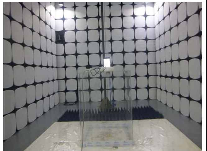
Radiated Spurious Emissions Test Setup Above 1GHz
