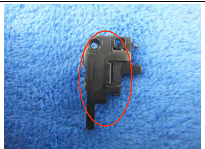
WIFI/BT/BLE/GPS - Antenna View
