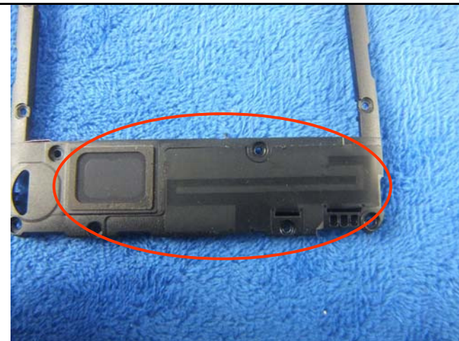
GSM/PCS/UMTS-FDD Antenna View
