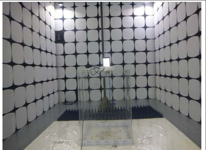
Radiated Spurious Emissions Test Setup Above 1GHz
