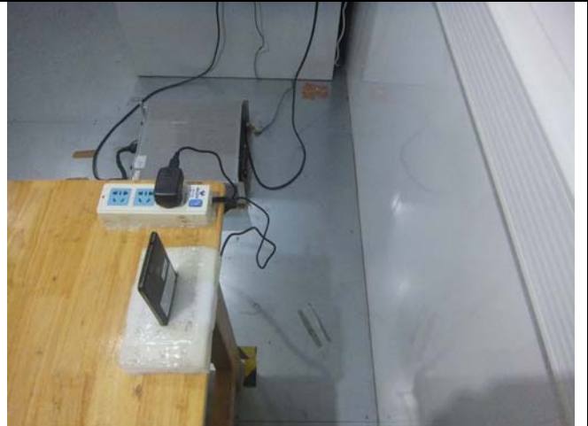
Conducted Emissions Test Setup Side View
