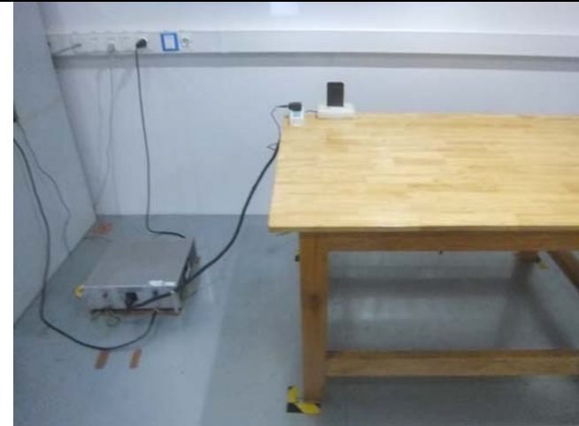
Conducted Emissions Test Setup Front View
