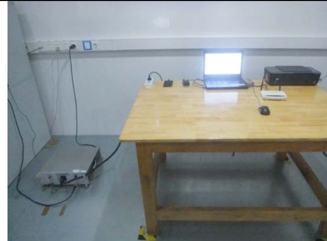
Conducted Emissions Test Setup – Front View
