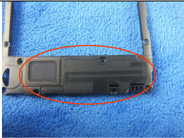
GSM/PCS/UMTS-FDD Antenna View
