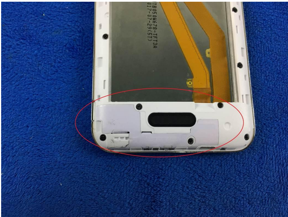
GSM/PCS/UMTS-FDD Antenna View
