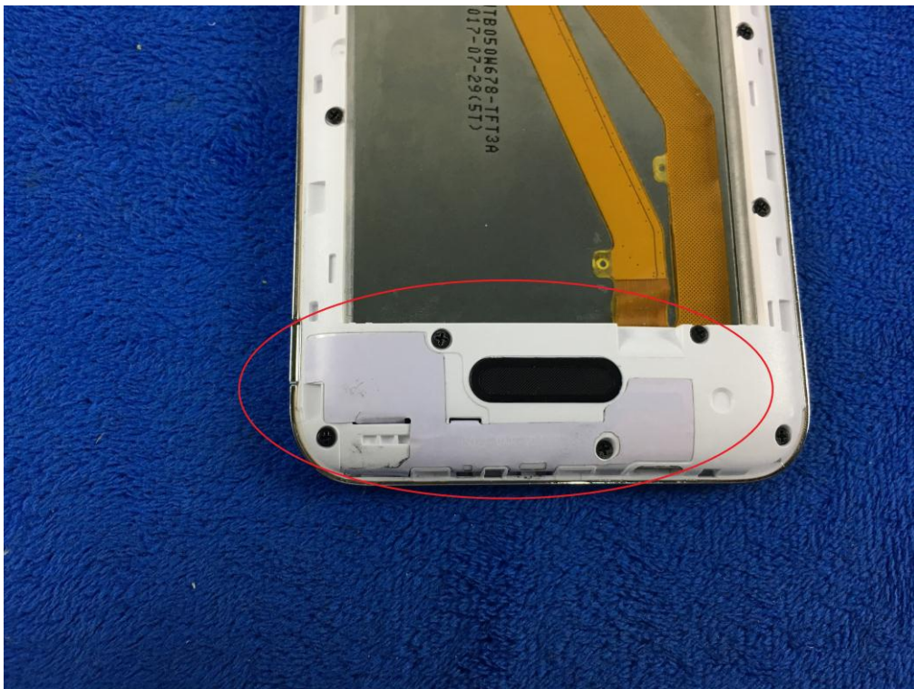
GSM/PCS/UMTS-FDD Antenna View
