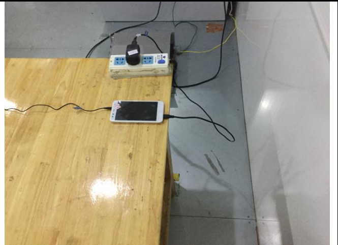
Conducted Emissions Test Setup Side View
