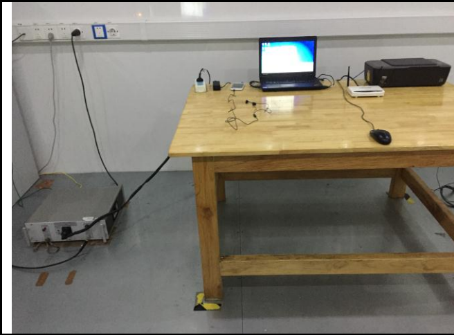
Conducted Emissions Test Setup – Front View
