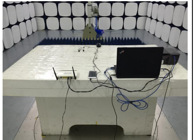
Radiated Emissions Test Setup Above 1GHz
