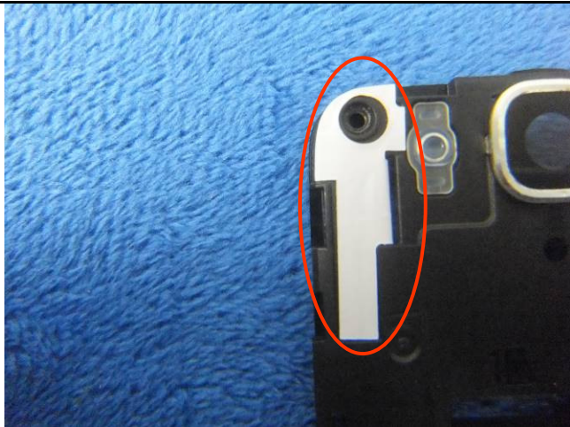
LTE Antenna View
